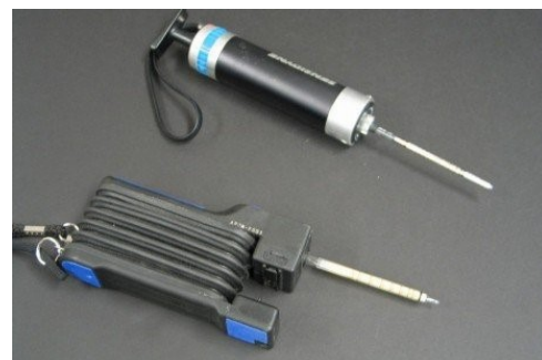
Examples of pull tube with pump for gas concentration detection.
