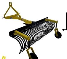
Some york rakes come with an option of **caster wheel** attachments. This allows the York rake to "float" and will help keep the York rake level when driving over uneven ground. York rakes can also have the option to be angled. This allows debris such as rocks to be pushed aside in and left in a wind row for easier clean up.
